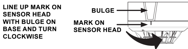
Figure 2: Attaching Sensor Head to Base
