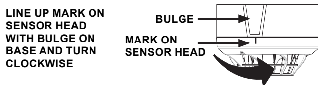
Figure 2: Attaching Sensor Head to Base
