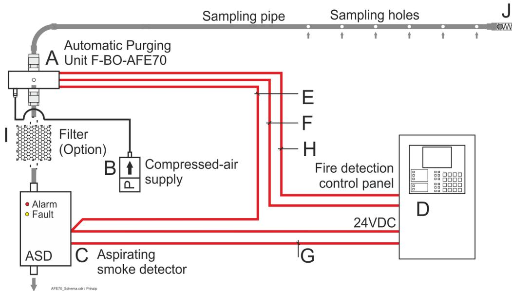
Fig. 2: Depiction of the structure of a system with an Automatic Purging Unit F-BO-AFE70 as well as the required components and connections
