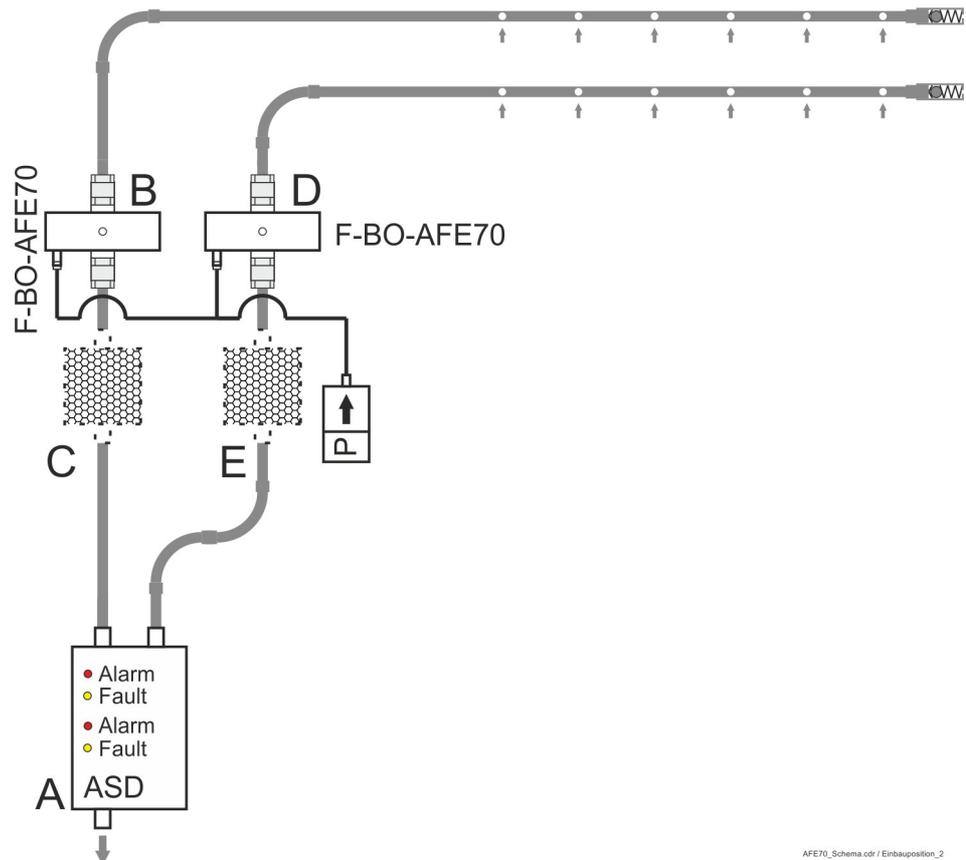
Fig. 8: Aspirating smoke detector with two separate pipe systems. As a supplement to Fig. 2 (page 10), electrical connection cables are not shown here in order to provide a clearer overview.
