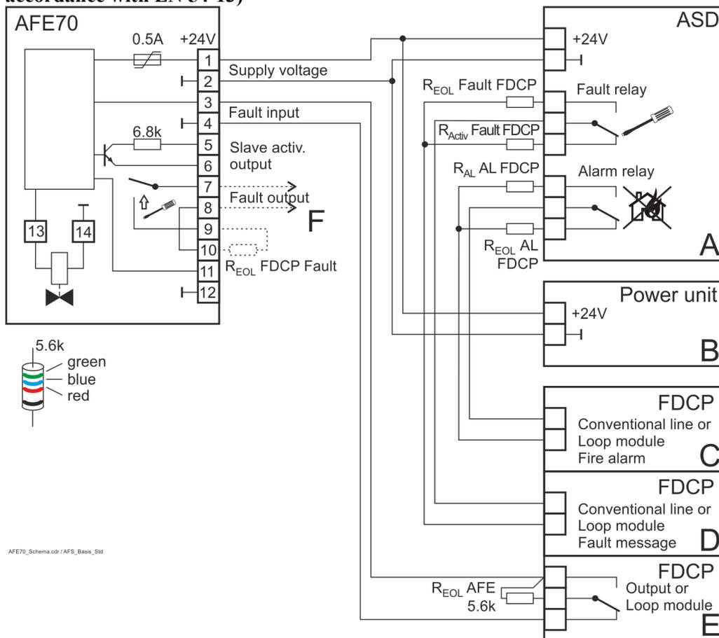
Fig. 12: Standard connection of the Automatic Purging Unit F-BO-AFE70 to the FDCP and to an ASD, via a monitored line. All components are only shown as schematic diagram, with the exception of the Purging unit.
