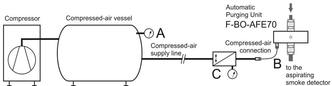
Fig. 3: Typical construction of a compressed-air system for providing the required compressed-air volume of an Automatic Purging Unit Series F-BO-AFE70, and explanation of the terms used in this chapter and by the calculation tool.
