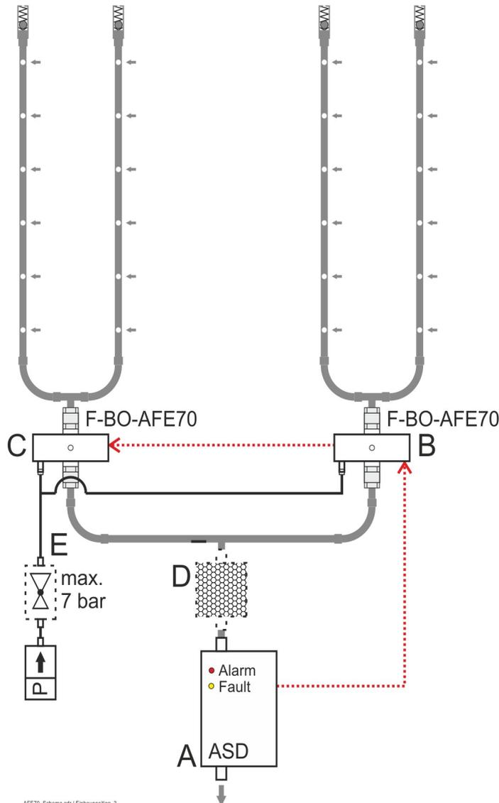
Fig. 9: ASD with one pipe network and two F-BO-AFE70's in master-slave arrangement. In the example, two F-BO-AFE70's are needed because of the total aperture area of the aspiration holes.
