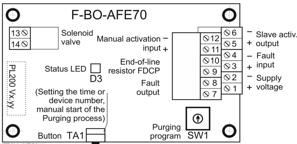
Fig. 11: Location of the display and operating elements and terminals on the control board AFS70-1 of the Automatic Purging Unit F-BO-AFE70
