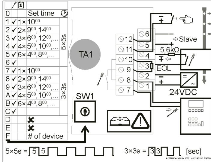
Fig. 16: Label showing the possible Purging programs, the location of the display and operating elements and the location of the terminals.
