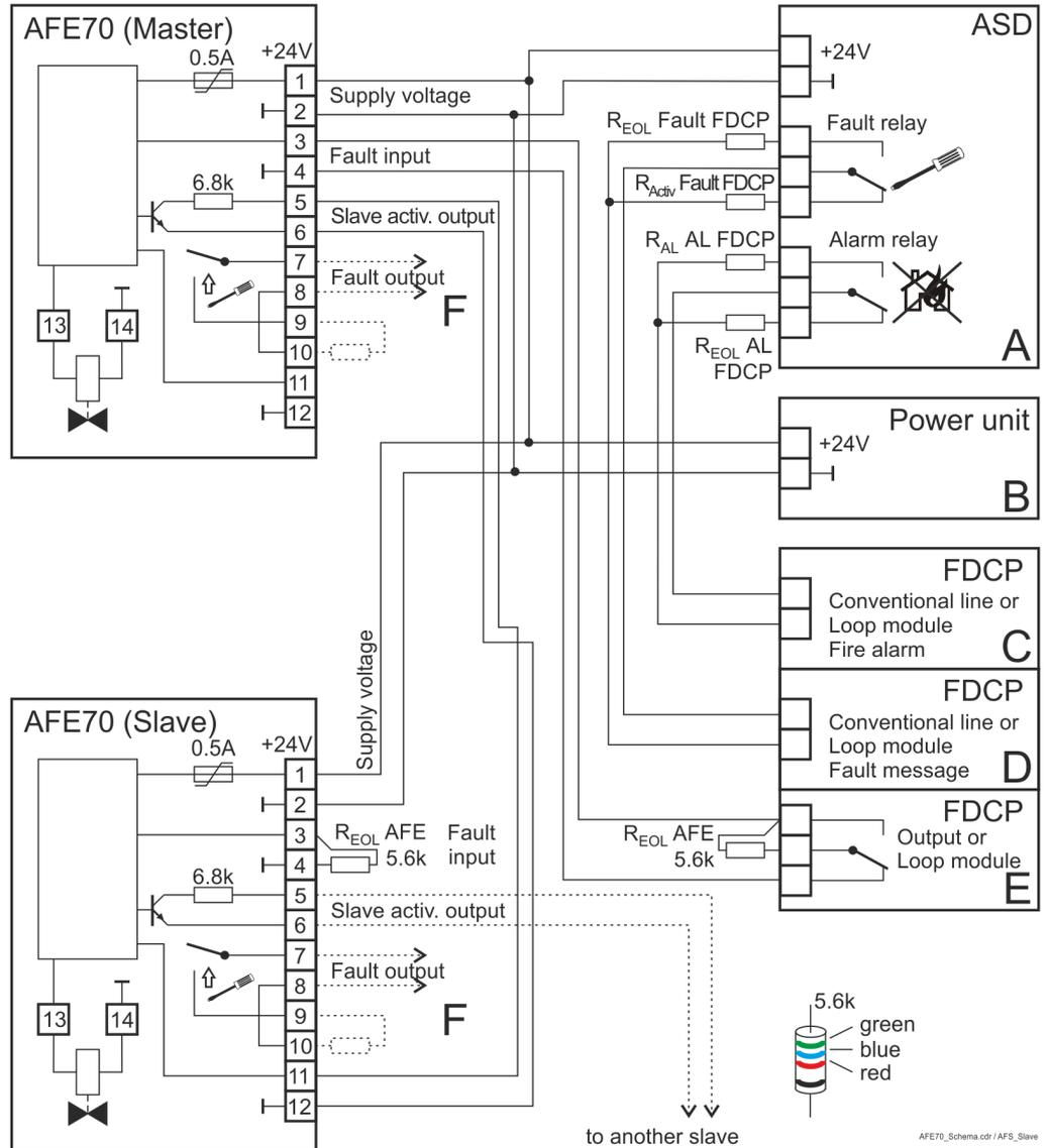
**Fig. 13:** Connection of two Automatic Purging Units F-BO-AFE70 in the master-slave mode.
