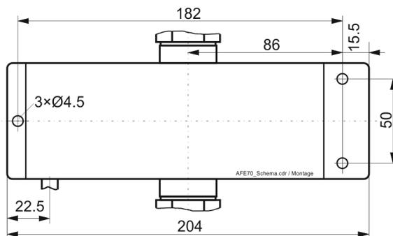
Fig. 7: Schematic illustration of the mounting holes and of the location of the connections for the sampling pipes and for the compressed air on the Automatic Purging Unit F-BO-AFE70
