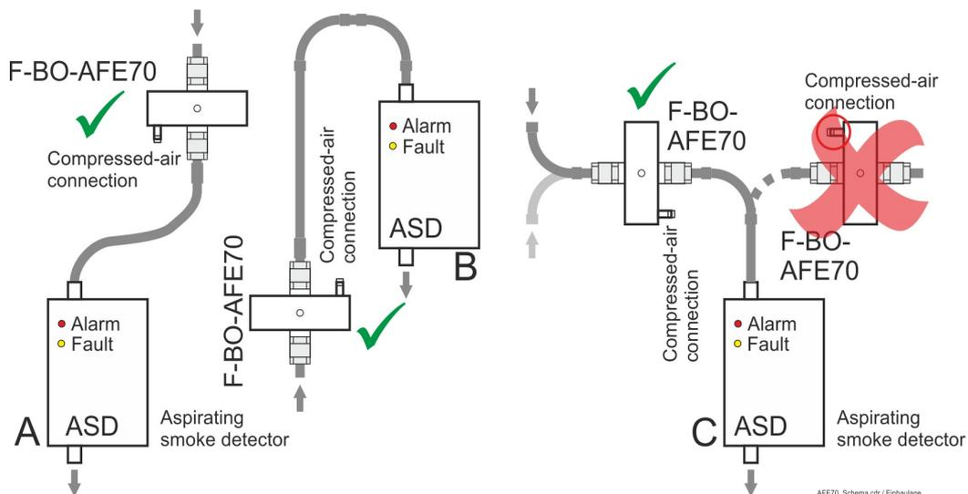
Fig. 6: Schematic illustration of the permissible wall mounting positions of the Automatic Purging Unit F-BO-AFE70 together with the evaluation unit and the pipe system of the aspirating smoke detector.
