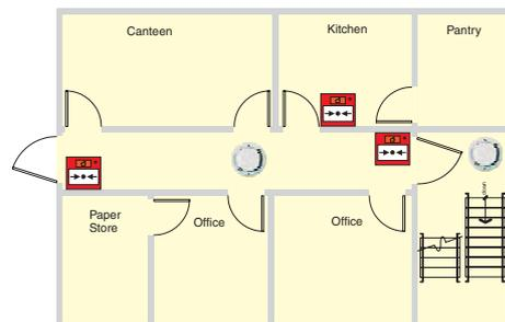
**Category L3:** Intended to offer early enough notification of a fire to allow evacuation before escape routes become smoke logged. Protection should be as for category L4 with the addition of smoke or heat detectors in rooms opening onto escape routes.
