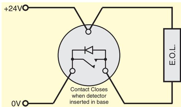
Fig 1.4.2. Active End of Line Monitoring Circuit
