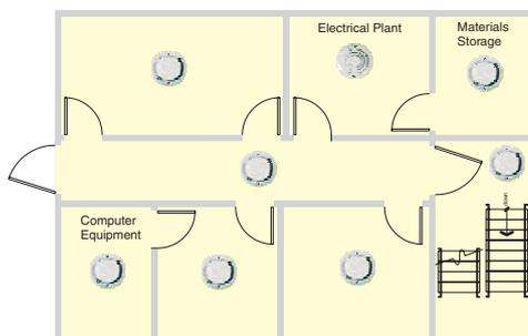
**Category P1:** The objective of a category P1 system is to reduce to a minimum the time from the ignition of a fire to the arrival of the fire brigade. In a P1 system, fire detectors should be installed throughout a building.
