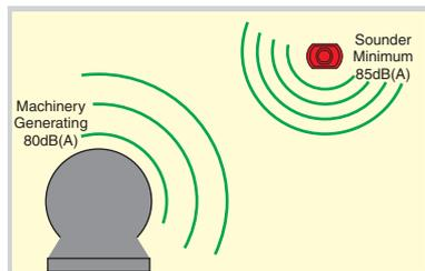
Where the alarm is intended to wake people, an SPL of 75dB(A) is required at the bed head. Generally this will require a sounder to be placed within the room.
