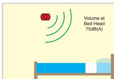
Where it is not possible to place a sounder within a room, there will be a loss of approximately 20dB(A) through a standard door, and 30dB(A) through a fire door.
