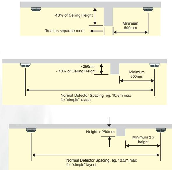
Figure 2.4.3: Detector Spacing around isolated ceiling obstructions
