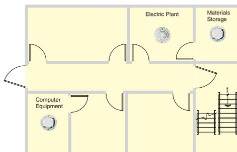
**Category P2:** Intended to provide early warning of fire in areas of high hazard, or to protect high-risk property. Automatic fire detection should be installed in defined areas of a building.
