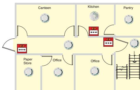
**Category L1:** The highest category for the protection of life. Intended to give the earliest possible notification of a fire in order to allow maximum time for evacuation. Automatic and manual fire detection installed throughout all areas of the building. Smoke detectors should be employed wherever possible to protect rooms in which people can be expected to be present.
