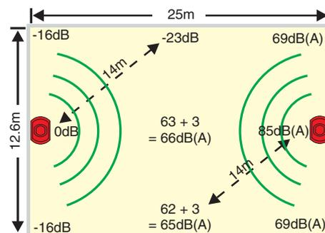
Note: dB(A) figures are for example only. Left side represents attenuation; right side indicates typical sound pressure level
