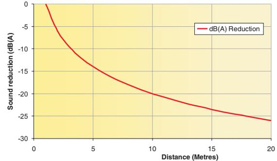
In open space, as the distance from a sounder doubles, the sound level will be reduced by 6dB(A), as shown.
