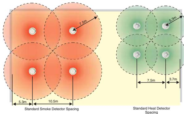
Figure 2.4.1: Simple spacing plans for smoke and heat detectors
