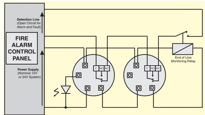
Figure 1.4.3. Typical 4 Wire System Wiring
