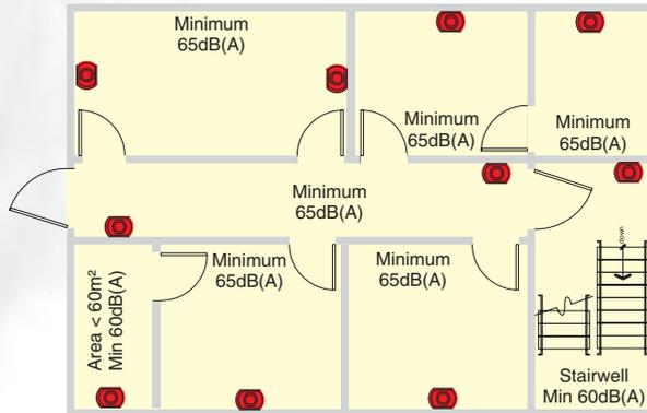
Figure 2.5.1. General Fire Alarm Sound Pressure Levels
