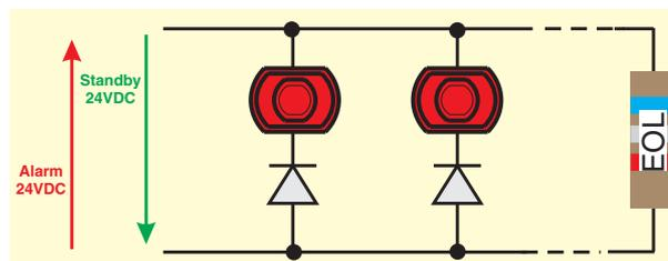
Figure 1.4.5. Conventional Fire Alarm Sounder Circuit
