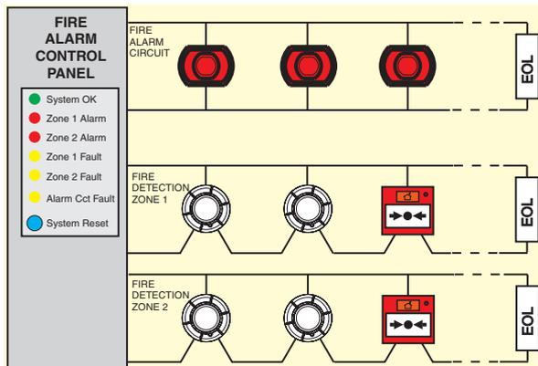
Figure 1.1: Simple Conventional Fire Alarm System
