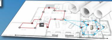
Figure 2 – Mesh Network: What happens if a communication link breaks in a mesh network
