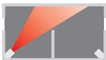
Without Smoke: Chamber is designed so that light from the IR-LED does not reach the receiver
