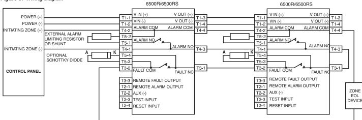
Terminals T5-1 and T5-2 provide connections used to complete the alarm circuit. A 0 ohm shunt, or current limiting resistor should be fitted depending on the application; these are supplied separately. Refer to the panel manufacturer for correct current limiting resistor values.
