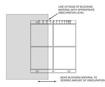
Figure 10. Reflector Test Card Procedure
