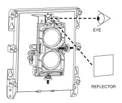
Figure 8: Coarse Alignment Procedure
