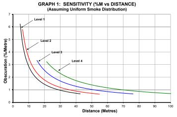
Total obscuration can be converted to percent per metre assuming uniform smoke density for the entire length of the beam. Graph 1 converts total obscuration to percent per metre for all acceptable sensitivity settings.
