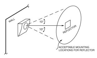
Figure 2a: Reflector Mounting Guidelines
