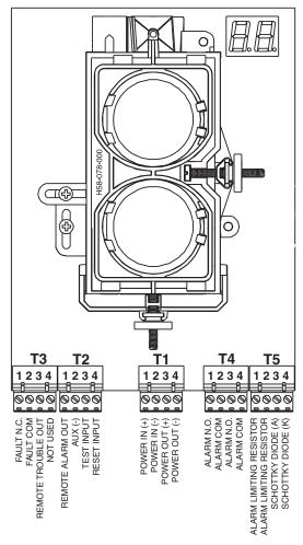
Figure 3: Detector Terminal Connections
