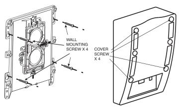
Figure 1: Transmitter/Receiver Wall Mounting
