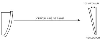
Figure 2b: Reflector Mounting Guidelines
