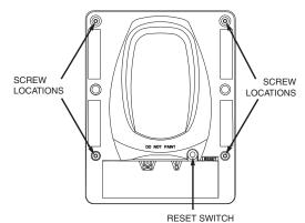
Figure 9: Housing Screw Locations
