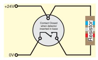
Figure 1.4.1. Resistive End of Line Operation
