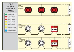
Figure 1.1: Simple Conventional Fire Alarm System
