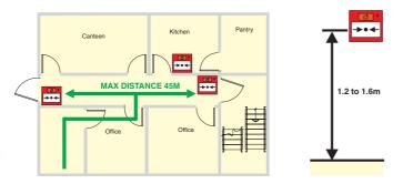
Figure 2.2.1. Manual Call Point Positioning
