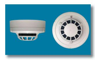
The 2351TEM photoelectric smoke/thermal detector incorporates an optical chamber and a thermal element, which in turn are continually monitored by the ASIC using algorithms developed specifically for the unit. An alarm signal is only enabled in the detector once the processor is satisfied that an incipient fire has been detected. By using a combination of inputs, the incidence of nuisance alarms is reduced whilst the response time to an actual fire is improved.
