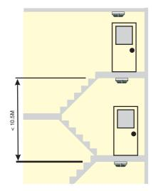
Figure 2.4.7. Detector in Stairwells
