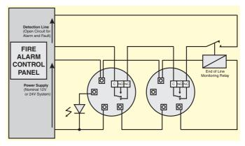
Figure 1.4.3. Typical 4 Wire System Wiring
