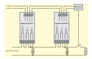
Figure 1.4.4. 4-Wire System with Full Monitoring
