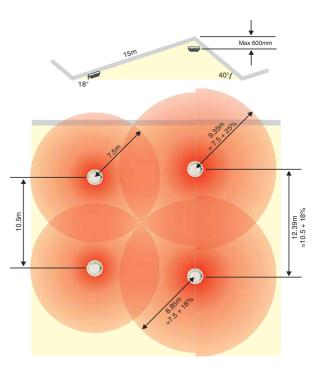
Figure 2.4.5. Spacing of Smoke Detectors under a Pitched Roof
