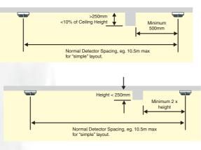
Figure 2.4.3: Detector Spacing around isolated ceiling obstructions
