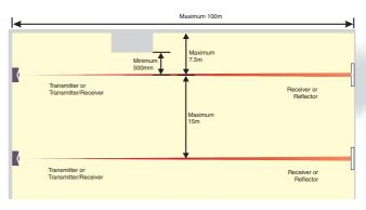
Figure 2.4.9: Standard Beam Detector Layout
