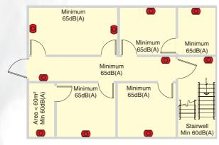
Figure 2.5.1. General Fire Alarm Sound Pressure Levels
