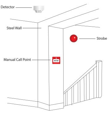
In this arrangement the sounder-strobe could have been located on the wall opposite to the manual call point at a required height.
