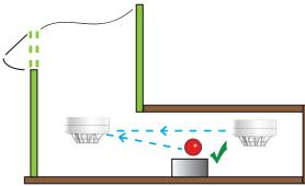
• **Don't** locate Agile<sup>™</sup> RF devices back to back where there is little or no attenuation, as 1m separation is required between RF devices
