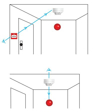
Figure 8: Example of Using the Line-of-Sight Technique
