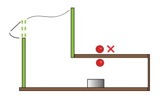
• **Don't** install gateways or Agile<sup>™</sup> RF devices near electrical switch gear
