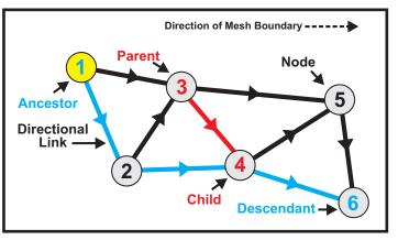
Note the unique and important Back-up Node #2; this has only one parent – the gateway. Its importance in the network is described below.
