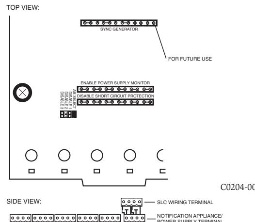
6. There is a power supply monitor that must be enabled to facilitate short circuit protection (see Figure 1). The module is shipped with power supply monitoring enabled represented by six large shunts on the pins of the "Enable Power Supply Monitor" area.
