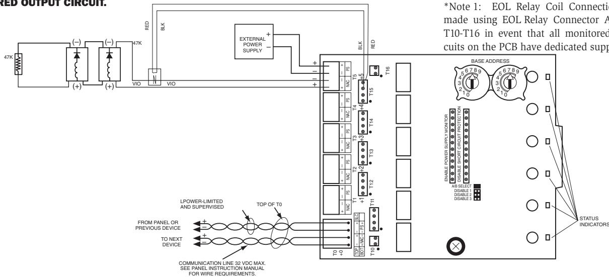
\*Note 1: EOL Relay Coil Connections must be made using EOL Relay Connector Assemblies on T10-T16 in event that all monitored Output Circuits on the PCB have dedicated supplies.
